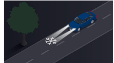
project markings on the road
